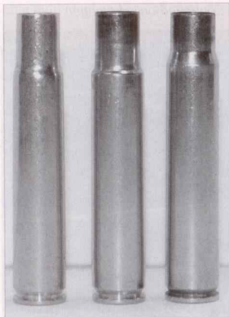
Case on left is a .35 Whelen, center is a .35 Whelen Ackley Improved and on right is a .358 Hawk. Note the extra body length of the Hawk round.
